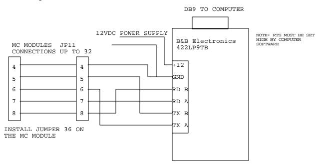
Note: Connecting RS-485 to a PC requires optional hardware (422LP9TB). The above diagram shows how to connect this optional hardware.
